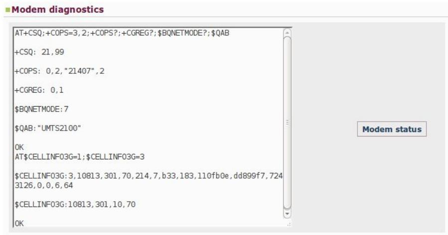
Fig. 30: Traces WWAN-1 – Modem diagnostics
